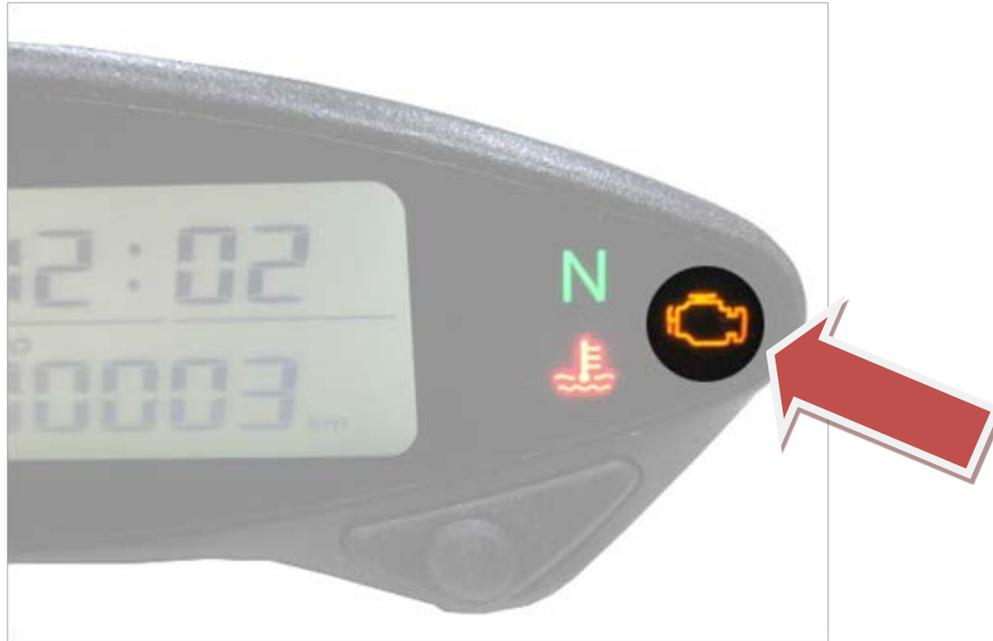
To know what is the fail and how proceed you can check the "On Board Diagnostic (OBD) Manual" that describes step by step how solve the errors show bu OBD tail light
