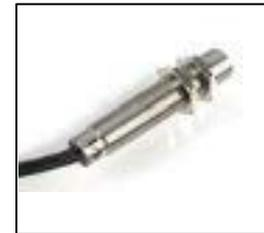
Wheel circumference pulses are different according to the type used. Hall sensors are 3 pulses per wheel and Reed sensors are 1 pulse.
