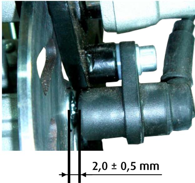
We can vary the distance with the help of a plastic washer until the correct distance is achieved . Verify that the distance is correct by checking the speed displayed on the clocks
