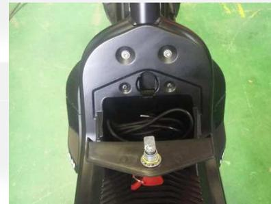
**2.- Remove the charging cable completely so that it is extended and connect the end to a household plug.**
